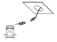
2. To connect the luminary to the network is by the use of a fast connector.
