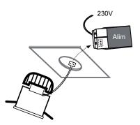
4.To connect the luminary to the food by the means of the connector envisaged for this purpose.
